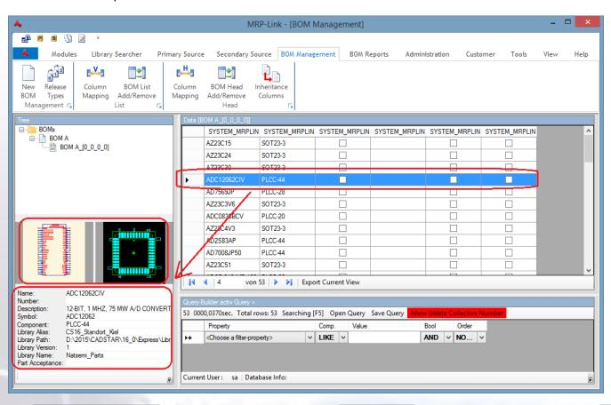
With a right index reference we will see inside the BOM Detailed View the SCM Symbol, the PCB Component and Part Details like (Part Name, Symbol Name, Library Alias, Library Path, Part Acceptance).
