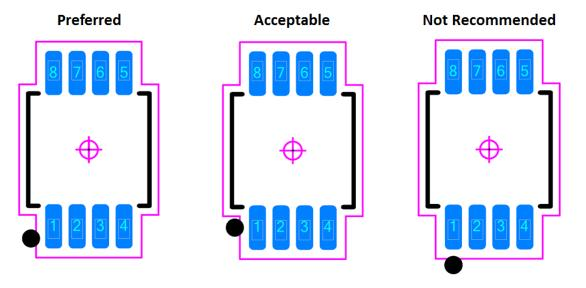
The component body outline legend line width should be a minimum of 0.125 mm. The Polarity Marking Symbol and component body legend should have a minimum 0.75 mm gap from the solder mask. The figure below illustrates the anatomy of a land pattern and feature sizes and spaces.
